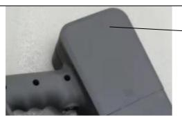
Here is the battery cover. The battery cover is opened by manually pressing the battery cover down and then opening the battery cover back.
